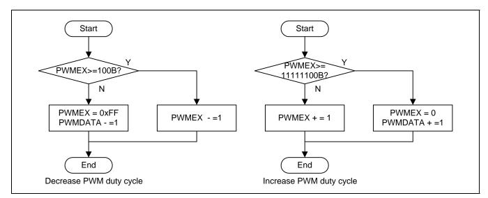
Figure 3-2 Way to change PWM duty cycle
